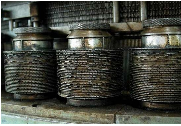
Wildt Mellor Bromley 9RJ36 Double Jersey Knitting Machine. This knitting machine has 36 ends of yarn feeding into the machine and is able to produce patterns up to four colours. The machine carries 1296 disks on 36 drums.
