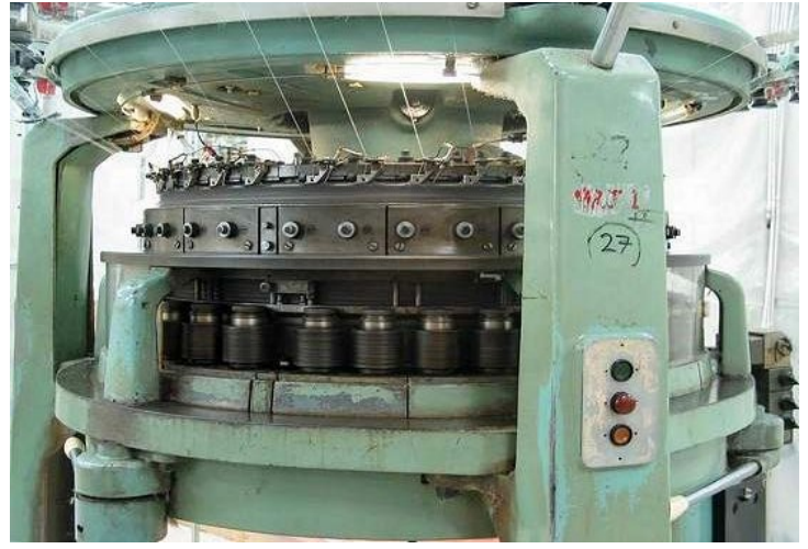
Wildt Mellor Bromley 9RJ36 Double Jersey Knitting Machine. This knitting machine has 36 ends of yarn feeding into the machine and is able to produce patterns up to four colours. The machine carries 1296 disks on 36 drums.
