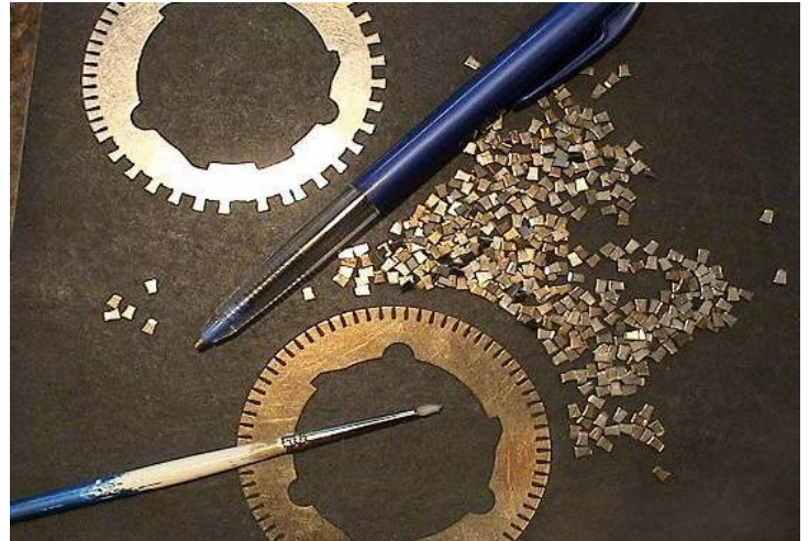
There are 72 teeth on an 18 gauge 9RJ disk. There are 84 teeth on a 22 gauge disk. The teeth are broken from the disks by hand one at a time. After breaking the teeth, the pieces are washed in white spirits.
