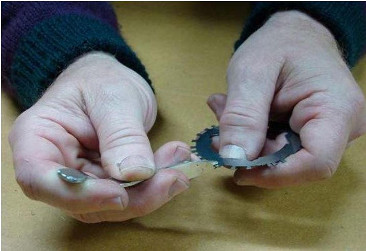
There are 72 teeth on an 18 gauge 9RJ disk. There are 84 teeth on a 22 gauge disk. The teeth are broken from the disks by hand one at a time. After breaking the teeth, the pieces are washed in white spirits.
